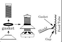
Position shield 3" above base to block rain from wetting feed.
